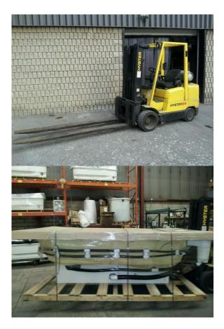
Do not remove packaging or skid until the tub is at its final location or unless it is absolutely necessary.
